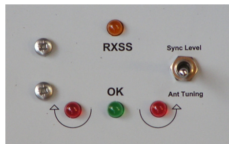
Fig 2. The antenna tuning indicator used to tune the antenna(s)
