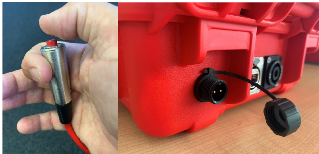
Fig 7. Optional external trigger button and panel port on the rear side of the Base.
